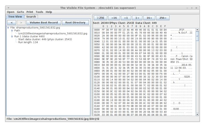
The file starts on data cluster 449 and has a run length of 134 data clusters. There is only one run, so the file is stored contiguously. The last data cluster is 449 + 134 - 1 = 582 (try to find it in the FAT!).
